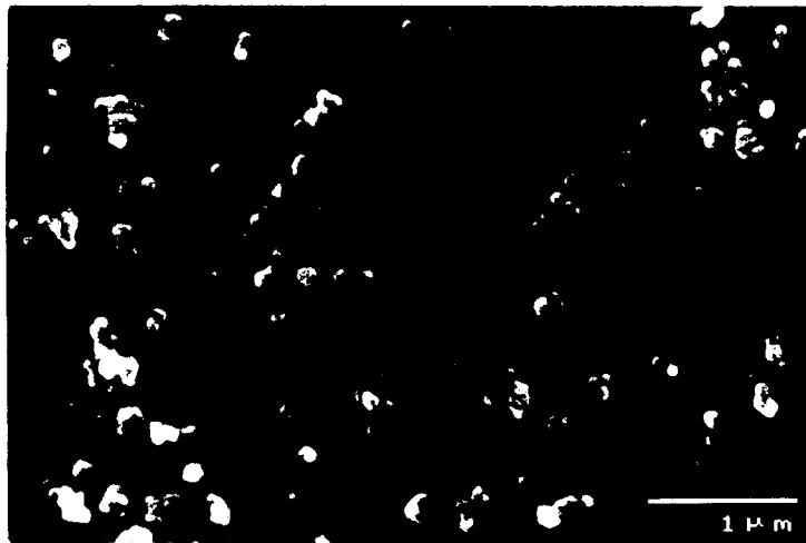
Fig. 5 SEM micrograph of particles in the LMZ from an etched specimen
