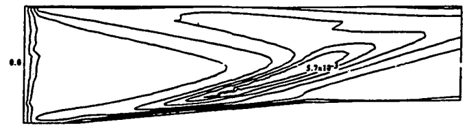
(j) OH Mass Fraction Contours (Max= 5.70 \times 10^{-3} , Min=0.0, \Delta=0.70 \times 10^{-3} )
