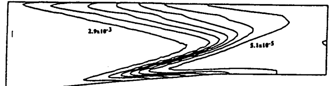
(h) H 2 Mass Fraction Contours (Max= 2.90 \times 10^{-3} , Min= 5.10 \times 10^{-5} , \Delta=3.60 \times 10^{-4} )
