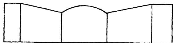
1 2 3 4 5 Intake Compressor Combustor Turbine Nozzle
