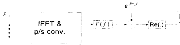
a) Basic structure of an OFDM Transmitter
