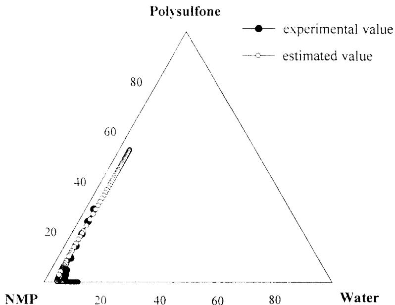
Fig. Comparision of experimental and estimated binodal curves for polysulfone/NMP/water system at 15°C
