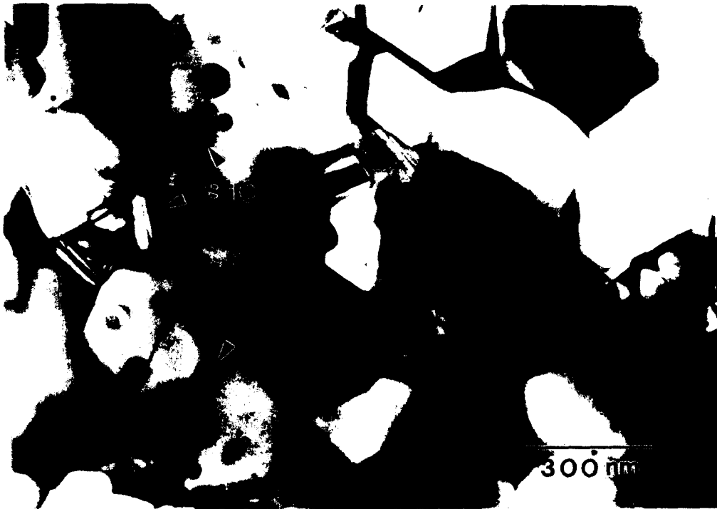
TEM micrograph showing that SiC particles are distributed both inside Si 3 N 4 grains and at grain boundaries.
