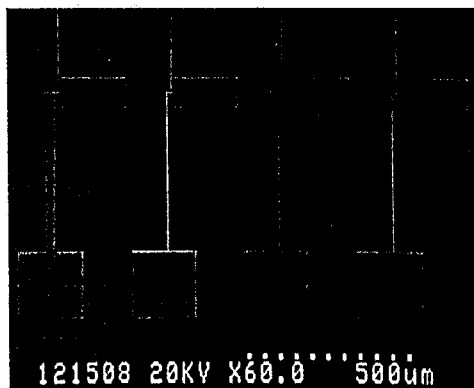
Fig.3 SEM photograph of the fabricated polysilicon micro actuator
