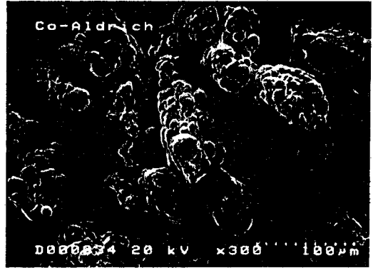
Fig. 2 SEM micrograph of Co skeleton sintered at 900℃, 2hr, H 2 atmosphere
