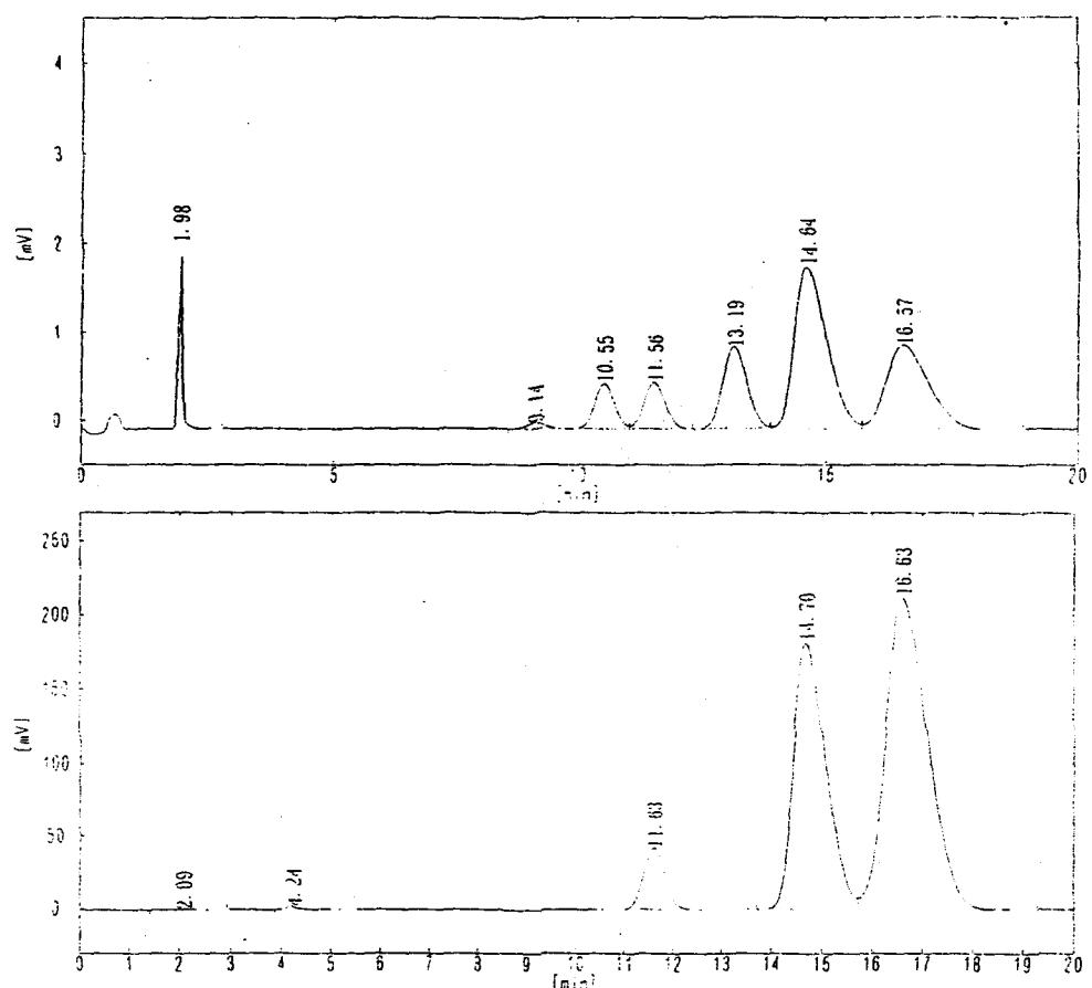
Fig. 2. Typical TCD and IC Responses of Helium and Hydrogen Isotopes.
