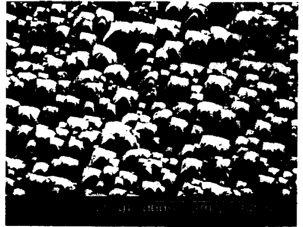
Fig.5. Pyramidally textured surface photographed by SEM (x1000, 30 ° tilted)
