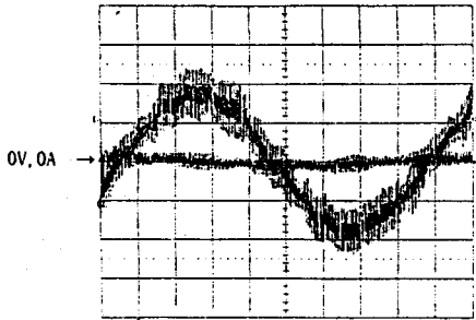
(a) at no load (100V/div, 5A/div, 2ms/div)
