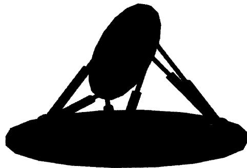
Fig. 4 Stewart Platform at  $\beta=63.5^\circ$
