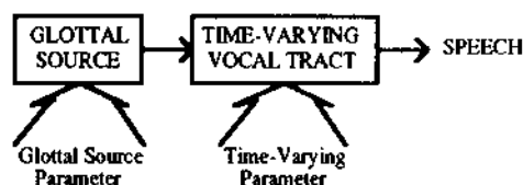
Fig. 1 Speech model using source-filter concept
