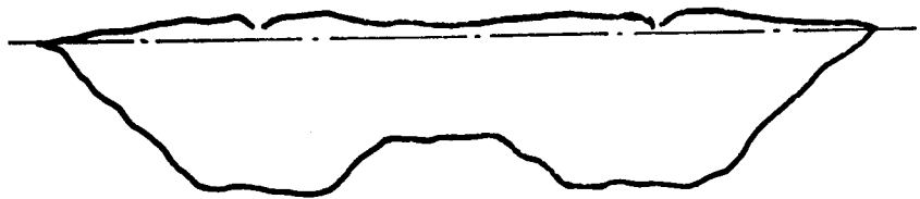
Fig. 6 Soil disturbance created by two winged subsoilers
