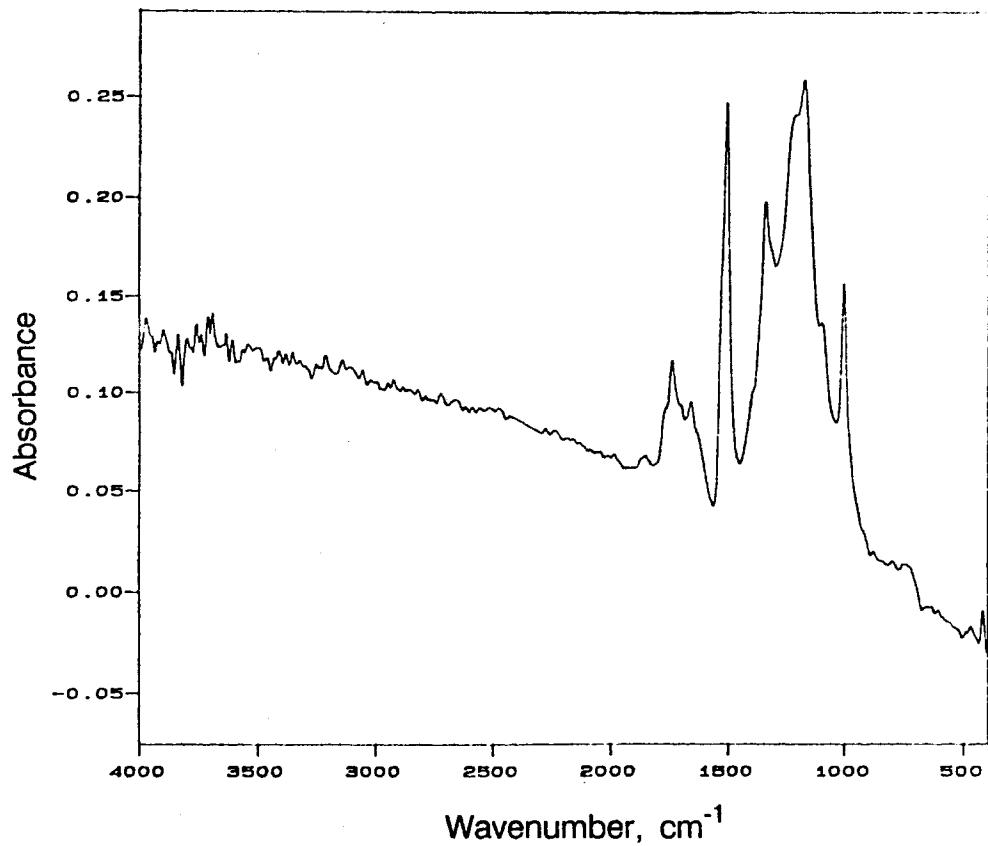
**Figure 1. FT-IR spectra of plasma - polymerized hexafluorobenzene.**
