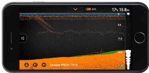
Fig. 11. Submarine topography obtained from Deeper CHIRP+.
