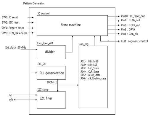
[Fig. 4] Proposed Pattern generation block structure
