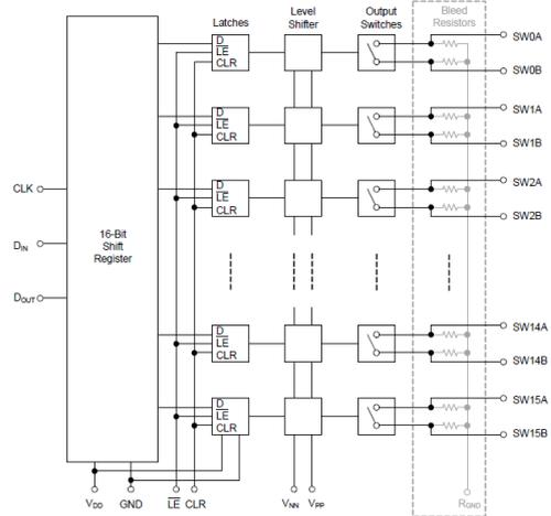
[Fig. 1] Multi-Channel Switch IC Structure
