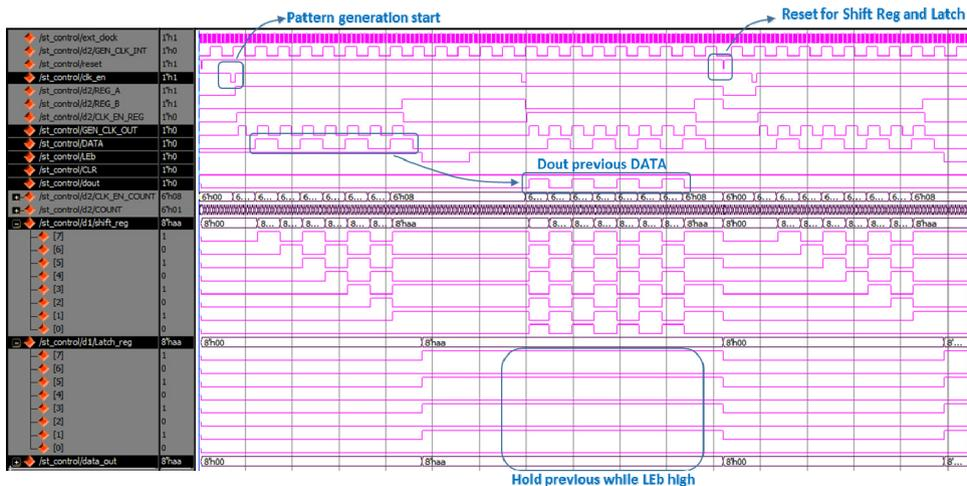
[Fig. 5] Simulation Waveform of Pattern Generation
