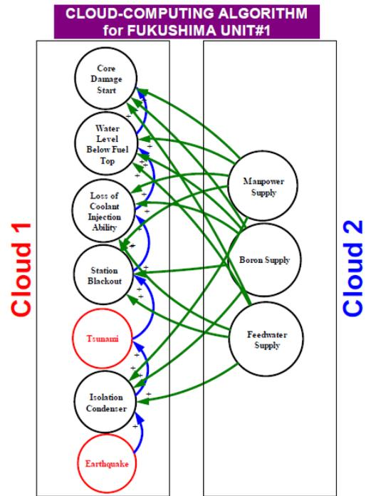
[Fig. 3] Diagram of reliability for Fukushima Unit1
