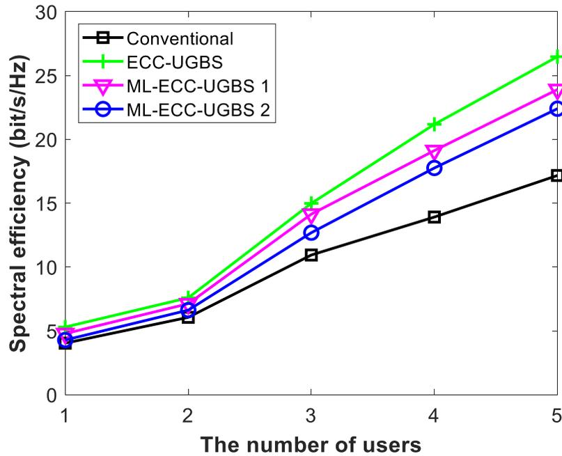
Figure 4. Spectral efficiency of conventional and proposed schemes versus the number of users (for SNR= 30 dB).
