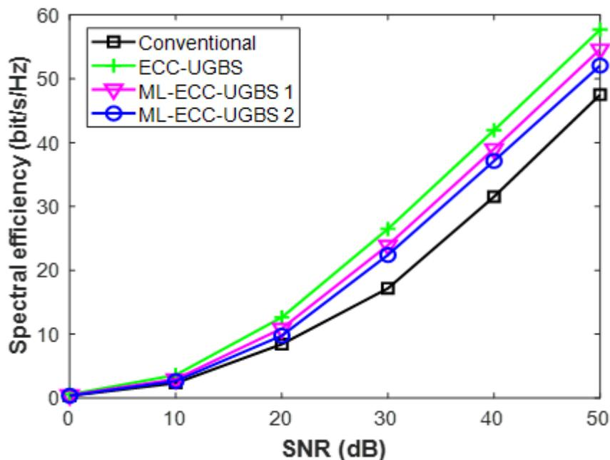
Figure 3. Spectral efficiency of conventional and proposed schemes versus SNR.
