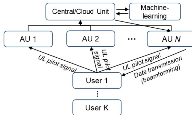
**Figure 1. A block diagram of the proposed coordinated mmWave system in multicell network.**
