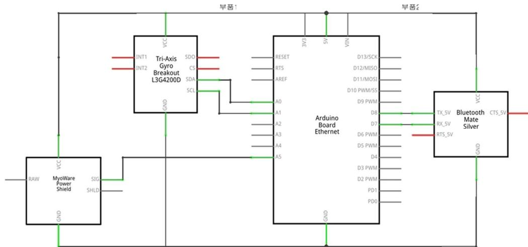
Figure 2. The Block diagram of System circuit
