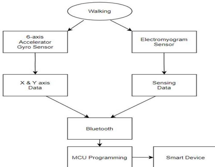
**Figure 1. Algorithm for gait measurement**
