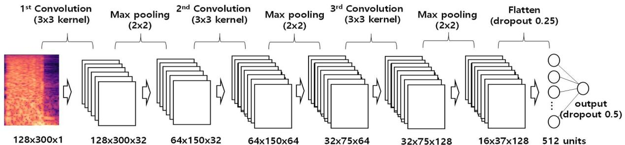
Figure 5. CNN model configuration for cough detection
