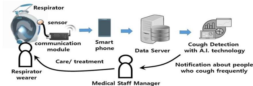
Figure 1. The overall structure of the cough detection system
