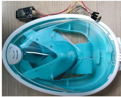
**Figure 2. Respirator and IoT devices**
