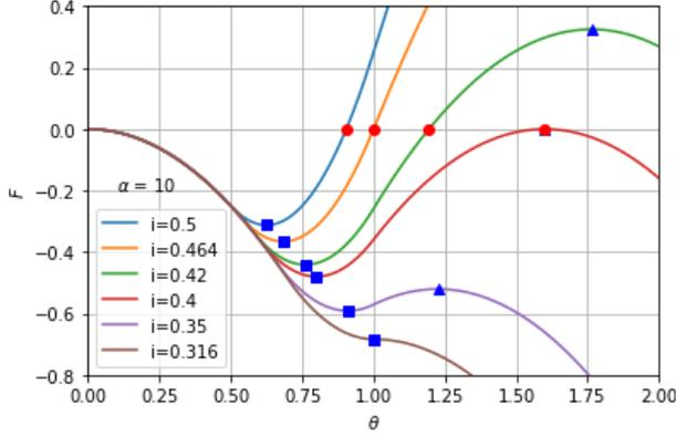
Fig. 2. Plot of stability function  $F(\theta)$  for Stekly parameter  $\alpha = 10$  with different current ratios.
