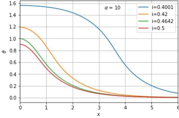
Fig. 3. Unstable equilibrium dimensionless temperature profile for Stekly parameter  $\alpha = 10$  and different current ratio  $i = I/I_c$ .
