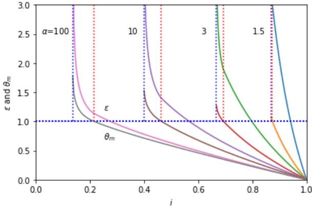
Fig. 4. A plot of dimensionless formation energy  $\epsilon$  and dimensionless maximum temperature  $\theta_m$  of the MPZ plotted against  $i = I/I_c$  with the Stekly number  $\alpha$  as parameter.
