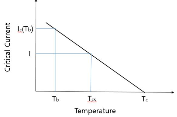
Fig. 1. Critical current vs. temperature.
