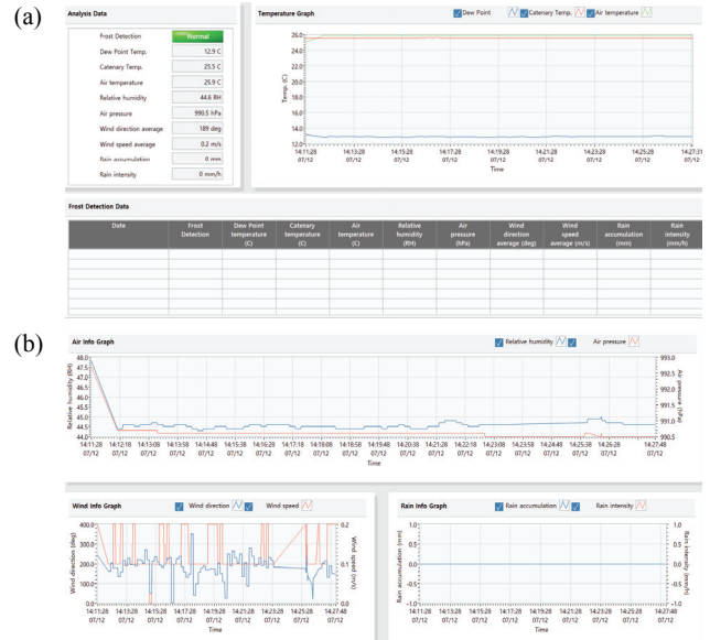
Fig. 5. The frost monitoring program of catenary system (a) analysis panel and (b) reference graph panel.
