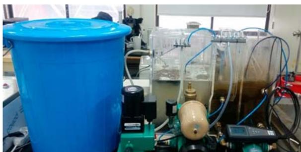
(A) Front view of the Bench-scale shipboard advanced wastewater treatment plant
