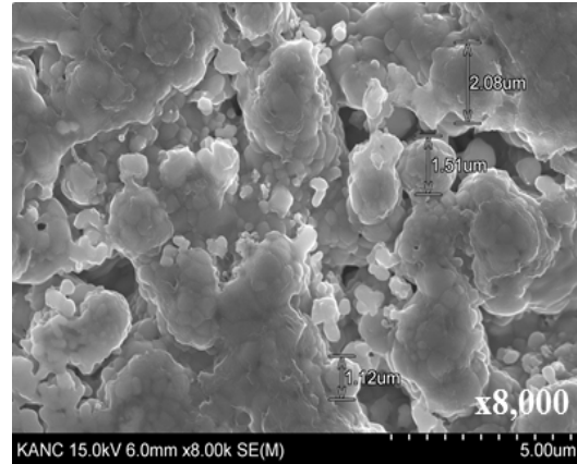
Fig. 2. SEM image of Ni-10%Ti-5%Ce-0.2%YSZ (ST-01) disk catalyst : ×8000.
