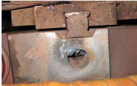
(b) Through-bolt end-region overheating, melting, and breakdown
