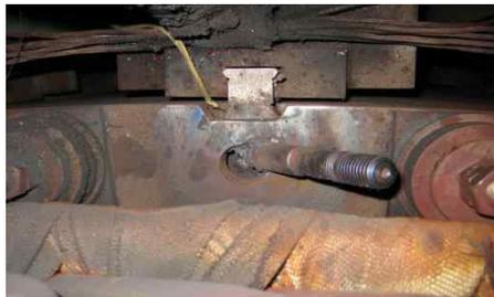
(c) Through-bolt end-region overheating and melting along with transverse fatigue fracturing
