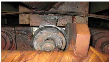
(d) Core bar overheating, with damaged bolt end-region showing significant greasy dirt buildup
