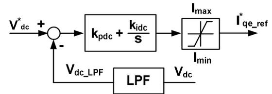
Fig. 5. DC link voltage controller
