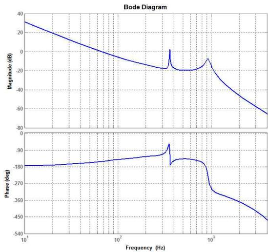
(a) Bode plot of open-loop transfer function
