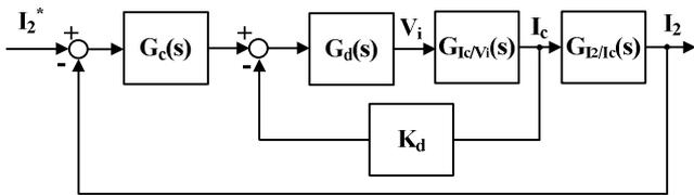
Fig. 11. Block diagram of current control considering active damping with capacitor current feedback
