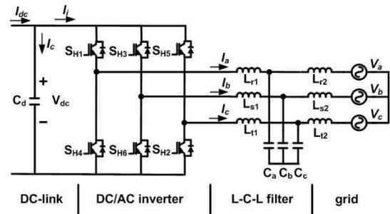
Fig. 4. Three-phase DC-AC inverter topology
