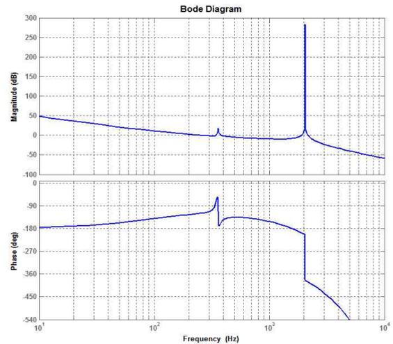
(a) Bode plot of open-loop transfer function
