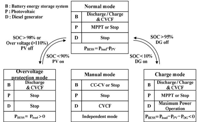
Fig. 3. Operation modes for stand-alone microgrid
