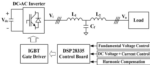
Fig. 2. Configuration of battery energy storage system
