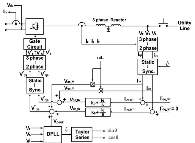
Fig. 6. DC-AC inverter current controller structure
