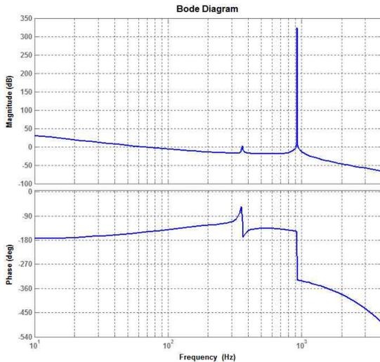
(a) Bode plot of open-loop transfer function
