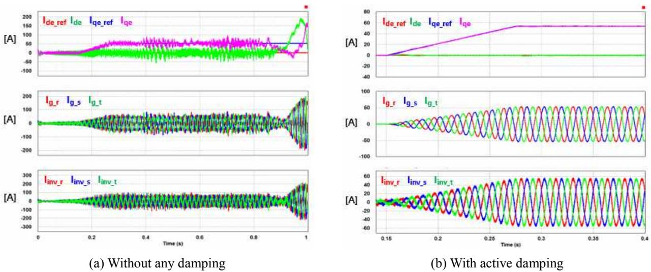
Fig. 14. Simulation results of BESS operations connected to diesel generator
