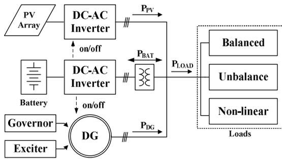
Fig. 1. Configuration of stand-alone microgrid
