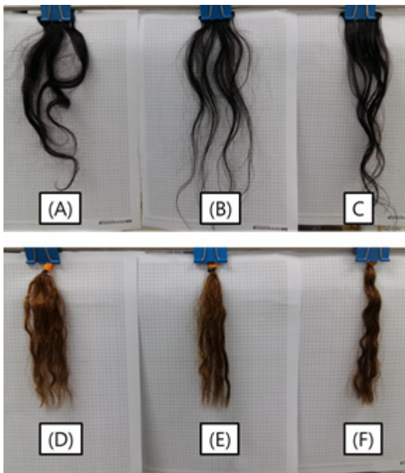
Figure 8. Test for flexibility with hair swatch treated by a shampoo formulated with a mixture of alkyl cellulose and guar gum. (upper) natural curly hair. (bottom) chemically permed hair. (A), (D) is curly hair swatch washed with 10% of SLES solution, (B), (E) treated with a shampoo composed of a cationic polymer, LR30M, (C), (F) treated with a shampoo composed of a mixture of alkyl cellulose and guar gum in a ratio of 3 : 1.
