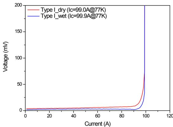
**Fig. 7.** Comparison of the test results between dry and wet winding conditions
