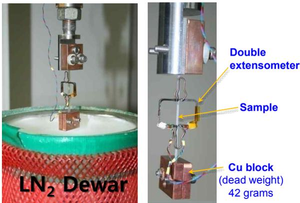
Fig. 3. Test setup for thermal strain measurement of the mixed epoxy resin and filler sample at 77 K
