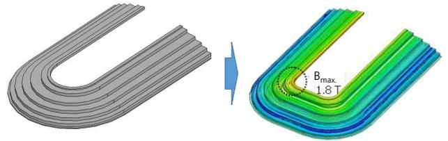
Fig. 2. Changing the shape of the coil end of the HTS field coil
