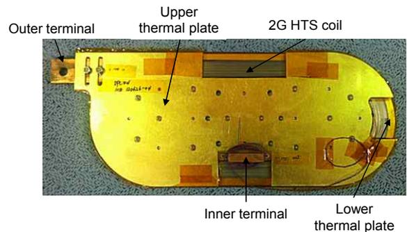
Fig. 5. Configurations of the small test coil
