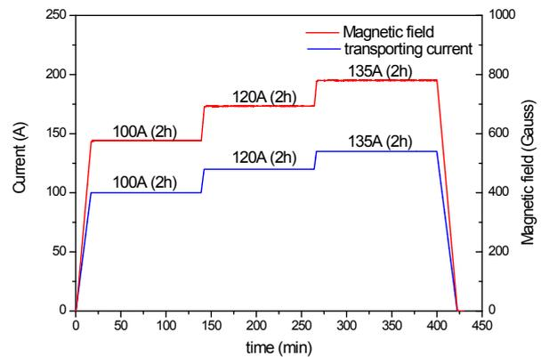
**Fig. 9.** Test results of the large test coil at 30 K conduction cooling
