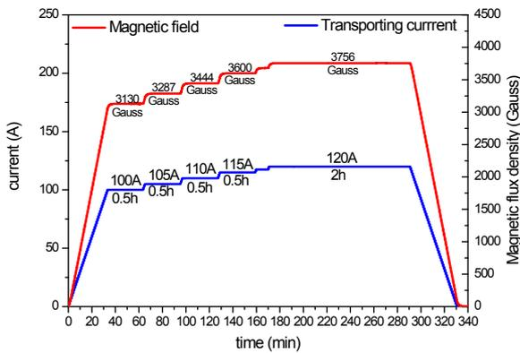
**Fig. 11.** Trend plot of the transporting current and magnetic field (at 30 K)
