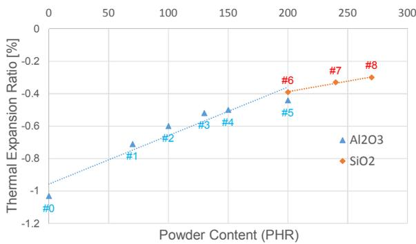
Fig. 4. Test results of the thermal expansion rate of the epoxy resin and filler sample
