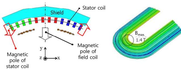
Fig. 1. Magnetic flux density distribution in the field coil
