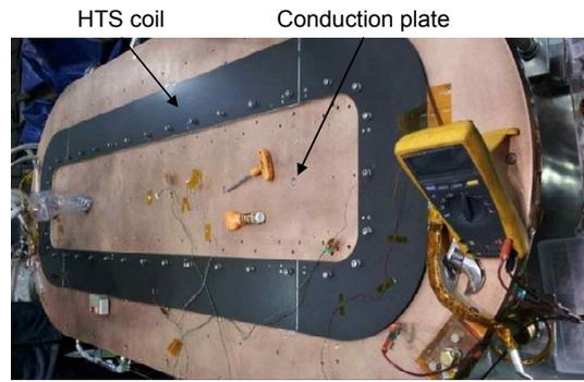
**Fig. 8.** A large 2G HTS test coil mounted on a conduction cooling test rig
