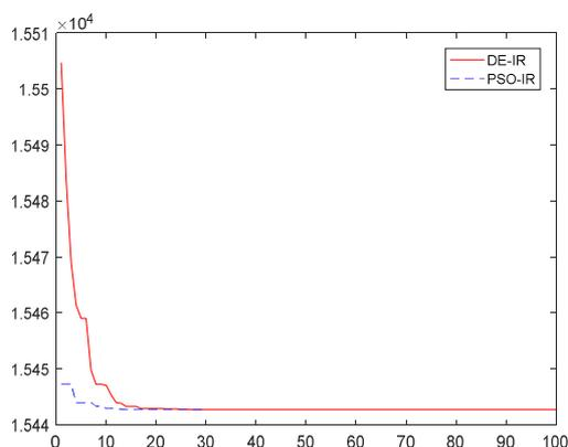
**Fig. 2.** Convergence of 6-generators system ( $P_D=1263\text{MW}$ )
