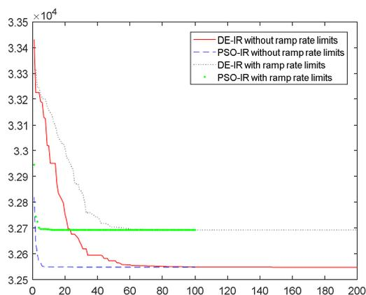
**Fig. 3.** Convergence of 15-generators system ( $P_D=2630\text{MW}$ )
