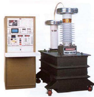
Fig. 1. Experimental equipment of partial discharge.
