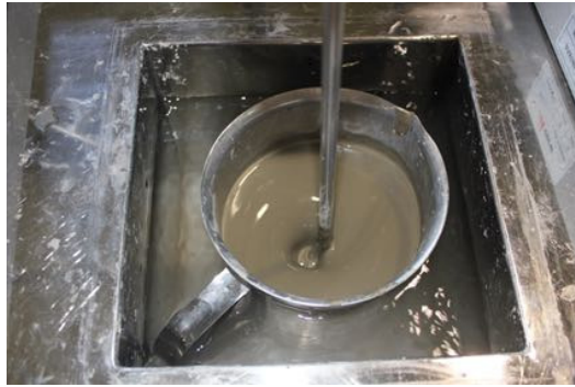
Fig. 4. Experiment to apply energy to grout in ultrasonic treatment bath
