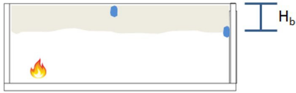
Figure 5. Installation places of beacons
