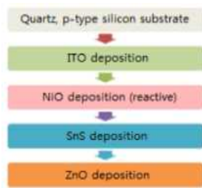
Fig. 1. Fabrication steps of n-ZnO/SnS/p-NiO/ITO/Quartz heterojunction photoelectric device.
