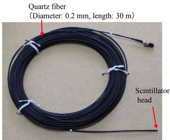
**Fig. 6.** Developed SOF detector consisting of the quartz optical fiber.
