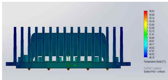
(b) LED module based on ADC-12 heat sink.
