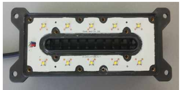
(a) LED module based on TCP heat sink.
