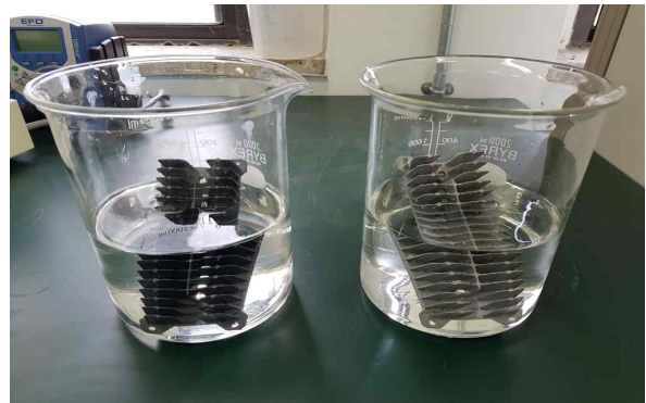
Fig. 4. Salt corrosion testing of heat sink.
