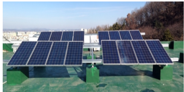
Fig. 1. Outdoor test bed of 4 kW PV modules (16 panels) on the roof of Cheonju Univ. Old Eng. Bldg. (E127°29'49", N36°39'9").
