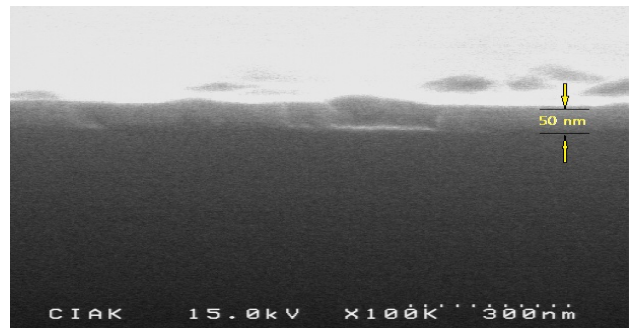
Fig. 4. SEM image of TiO 2 layer on SiC substrate.
