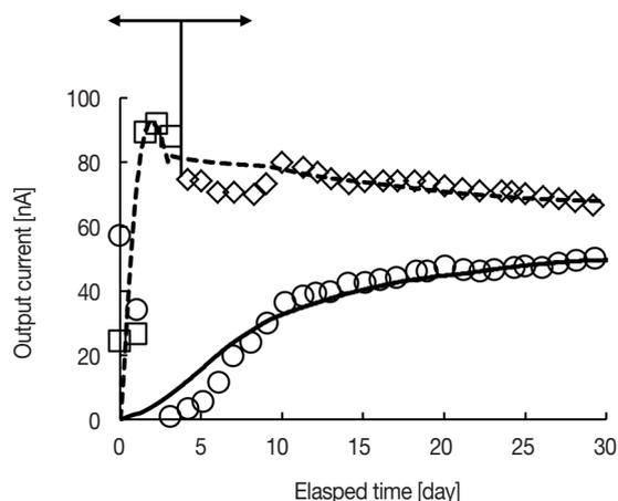
**Fig. 5.** The experimental data and the calculated results from electrochemical analysis. The calculated results are shown as solid line or dashed line reproduce the experimental data are represented by square.
