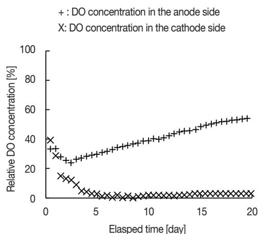
**Fig. 4.** Experimental data of DO concentration measurement. DO concentration in the anode side is increasing, whereas that in the cathode one decreasing.
