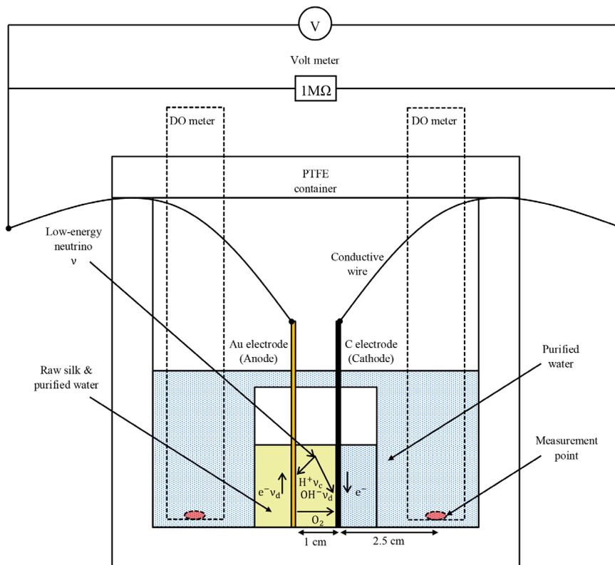
Fig. 3. Illustration of the low-energy neutrino detector. Raw silk arranged around an anode generates  $B^0$  field. When low-energy neutrino enters into this region, it is supposed to be dissociated into two constituent particles.
