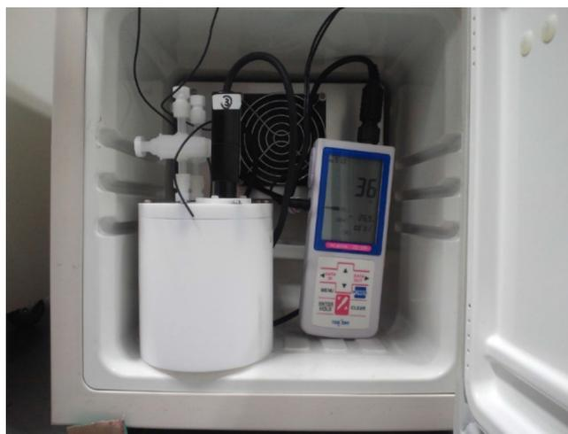
Fig. 2. Picture of the detector appearance and DO meter in incubator.
