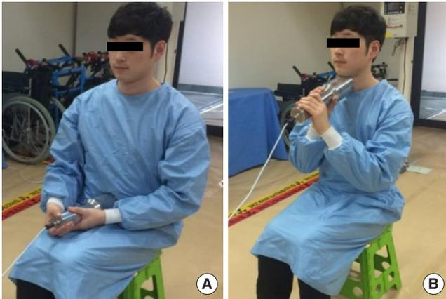
Fig. 1. Counting geometries for *in-vivo* monitoring: (A) Whole body counting and (B) Thyroid monitoring.
