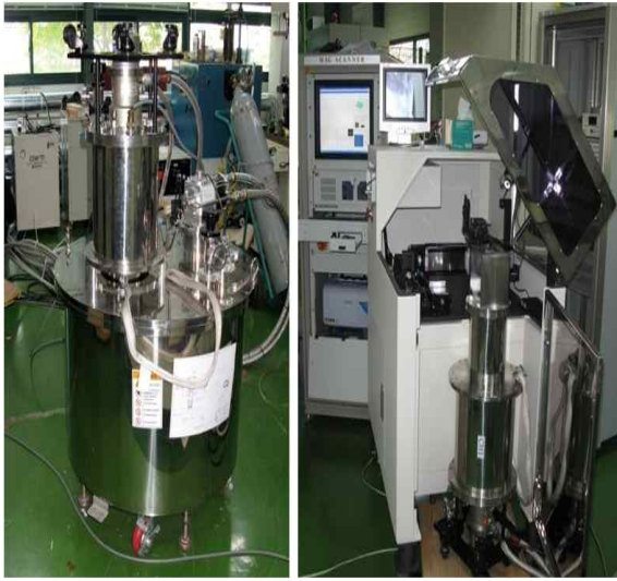
Fig. 7. Magnetization of superconductor bulk(left) and measurement of trapped magnetic field(right) by using 2 T class magnetizer.
