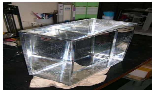
Fig. 3. Water slab phantom made by KRISS.
