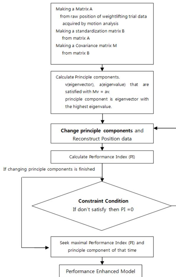
Figure 1. Procedure for calculation of Performance Enhanced Model
