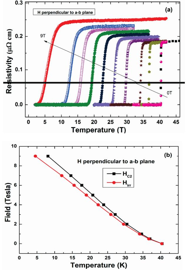
Fig. 3. (a) Resistivity transitions measured at various fields from 0 to 9 T when H was applied perpendicular to a-b plane of MgB<sub>2</sub> thin film. (b) Temperature dependence of  $H_{c2}$  and  $H_{irr}$ .
