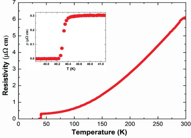
Fig. 1. Temperature dependence of resistivity for single-crystal like MgB<sub>2</sub> thin film grown on Al<sub>2</sub>O<sub>3</sub> substrate. The inset shows the magnified view of superconducting transition in the temperature region from 39 to 41 K.
