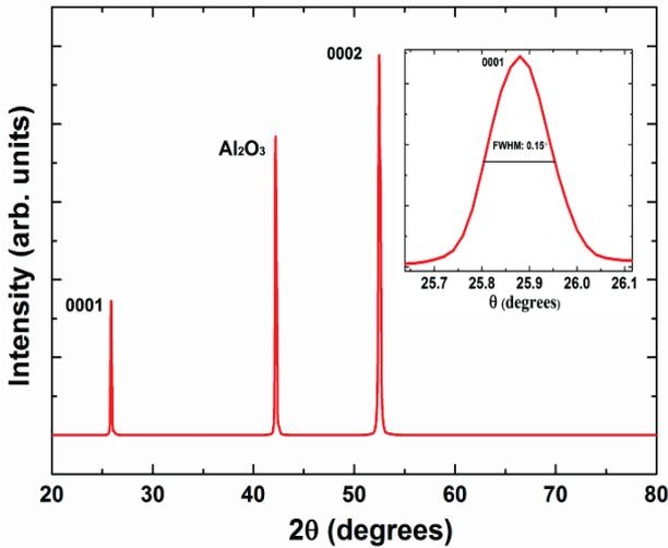
Fig. 2. The X-ray diffraction of single-crystal like MgB<sub>2</sub> thin film grown on (0001) Al<sub>2</sub>O<sub>3</sub> substrate. The inset shows the full width at half maximum (FWHM) obtained from the (0001) peak of MgB<sub>2</sub>.
