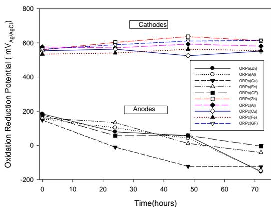
**Fig. 1.** Oxidation reduction potential (ORP) variations in the cathode and anode (against Ag/AgCl) in our sediment microbial fuel cell.
