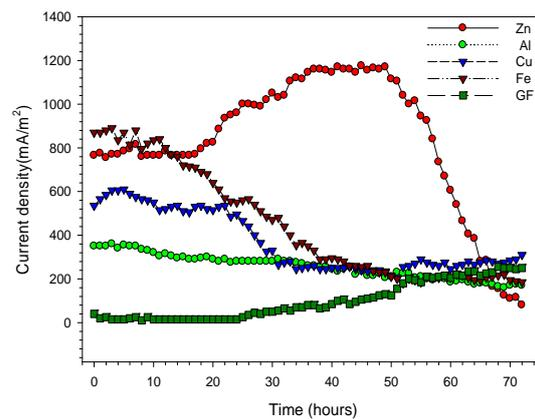
Fig.4. Current density vs time of SMFC operation (surface area 0.002 m<sup>2</sup> and internal resistance 20 $\Omega$ ).
