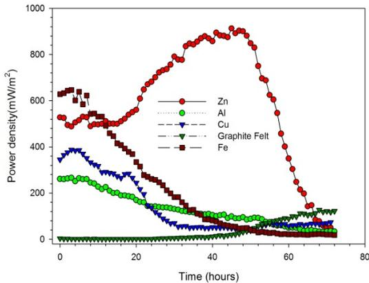
Fig. 2. Power density of SMFC according to different anode with respect to time.
