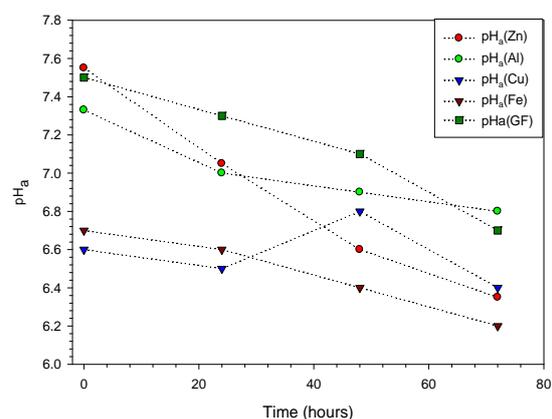
Fig. 5. pH changes in anode chamber over time of SMFC (pHa, anodic pH).
