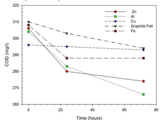
Fig. 6. Chemical oxygen demand (COD) in anode part decreasing with respect to time.
