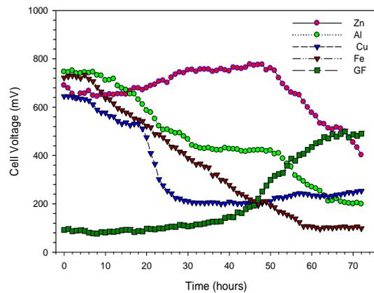
Fig. 3. Cell voltages of SMFC with respect to time.
