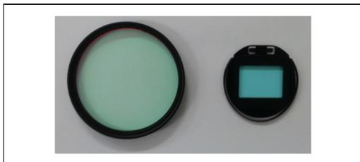
[Fig. 7] The adopted visible and near-infrared ray filter
