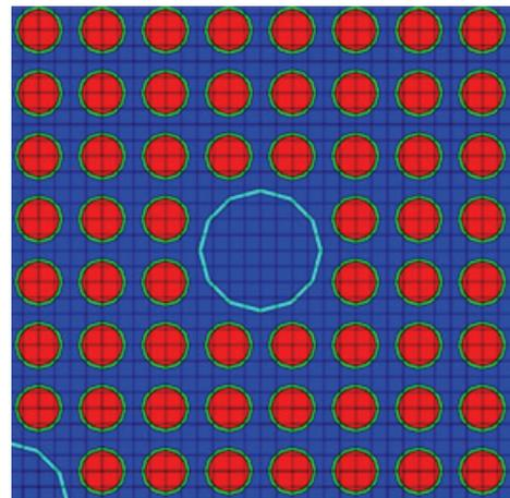
**Fig. 1.** A 1/4 fuel assembly model generated using the TRITON module.
