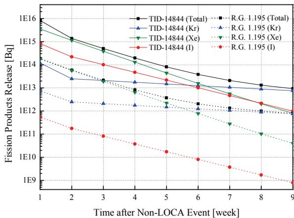
**Fig. 3.** Fission products released into the environment according to time after the non-LOCA event.
