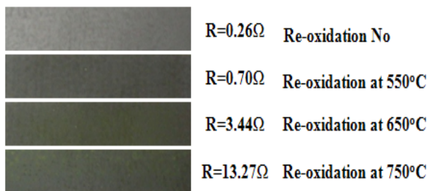
Fig. 3. Appearances and resistances of Ni-electrodes on alumina substrate re-oxidized at various temperatures after firing at 900°C for 2 h in reduced atmosphere of PO_2 = 10^{-6} Pa.
