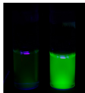
Fig. 6. Photographic images of 5 \mu\text{M} in methanol (left) and upon addition of 104 equiv. formaldehyde (right) under hand-held UV lamp ( \lambda_{\text{max}} = 365 nm).
