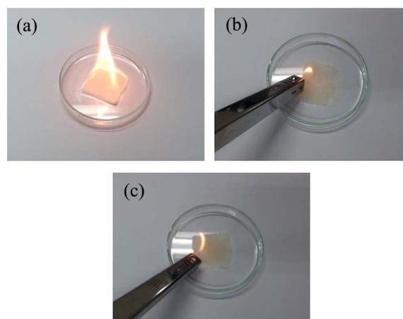
**Figure 7.** Photographic images showing the flammable behavior of different electrolyte systems during flammability test: (a) liquid electrolyte, (b) ionic liquid electrolyte and (c) ionic liquid-based gel polymer electrolyte.
