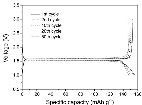
**Figure 4.** Charge and discharge curves of the Li<sub>4</sub>Ti<sub>5</sub>O<sub>12</sub> electrode in ionic liquid-based gel polymer electrolyte cured by 8 wt % of cross-linking agent (0.1 C rate, cut-off voltage range of 1.0-3.0 V, 55 °C).
