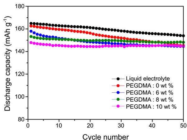
**Figure 5.** Discharge capacities as a function of the cycle number for the Li<sub>4</sub>Ti<sub>5</sub>O<sub>12</sub> electrode in different electrolyte systems (0.1 C rate, cut-off voltage range of 1.0-3.0 V, 55 °C).
