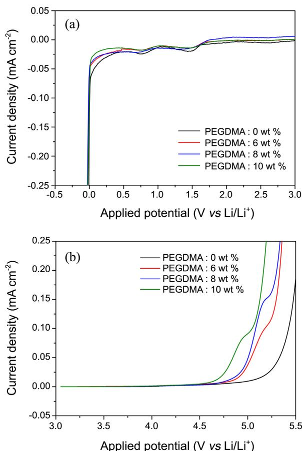
**Figure 3.** Linear sweep voltammograms of the ionic liquid-based gel polymer electrolytes cured with different amounts of cross-linking agent (scan rate: 1 mV s<sup>-1</sup>). (a) cathodic scan and (b) anodic scan.
