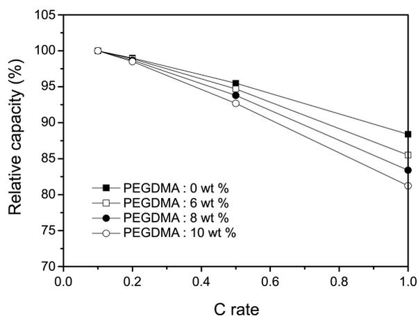
**Figure 6.** Relative capacities, as a function of C rate, of the  $\text{Li}/\text{Li}_4\text{Ti}_5\text{O}_{12}$  cells assembled with ionic liquid electrolyte and cross-linked gel polymer electrolytes cured by different amounts of cross-linking agent.
